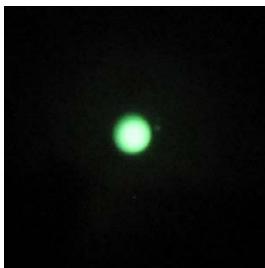
Figure 3. Field electron microscope image of the e-beam emitted from the CNT electron gun.
