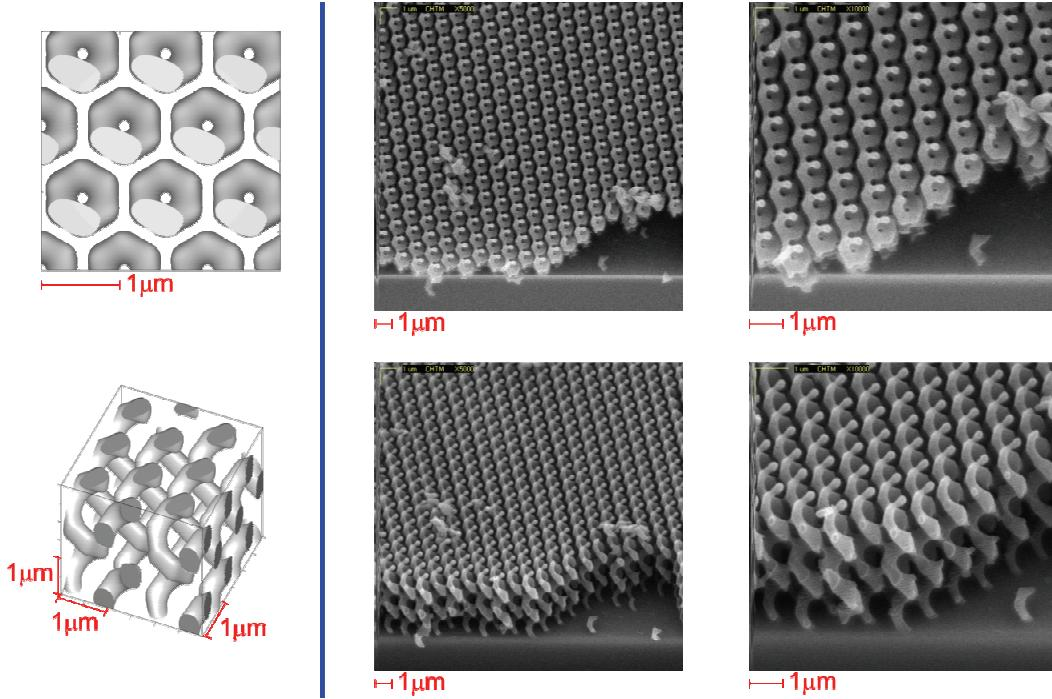
**3D helical photonic crystals fabricated using 6 two-beam exposures with 60° rotation (355 nm exposure, NR7 resist –  $n \sim 1.7$ ).**
