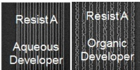
Figure 2. Resist A developed by Aqueous Developer (left) and Organic developer (right). Resist Patterning was performed at KrF
