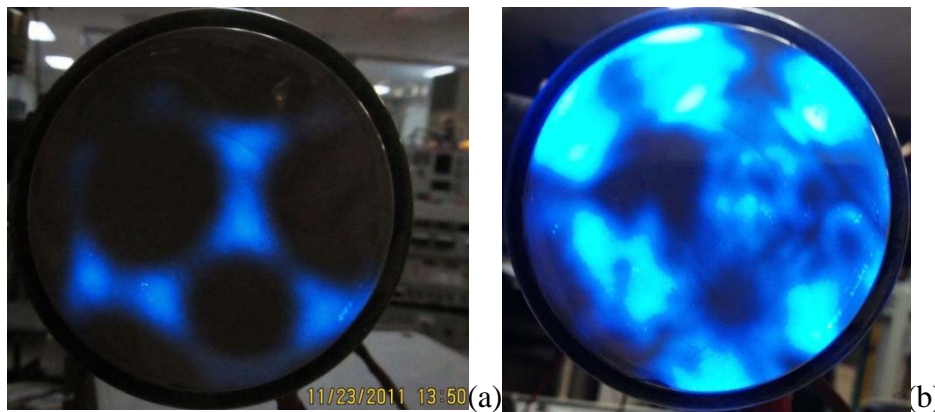
Figure 3: (a) A typical field emission pattern from HfC where the (310) planes are bright; emission level is \sim 10 \mu\text{A} . (b) The emission pattern after running for \sim 300 hours at 1500 K. Here the emission has increased to \sim 1 mA
