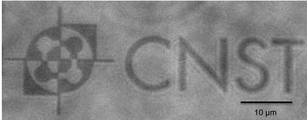
Figure 1: Optical Image of Li + -Implanted WO 3 Film: 2 keV Li + ions implanted using a magneto-optical trap ion source create localized optical absorption. Image acquired with 750 nm light.
