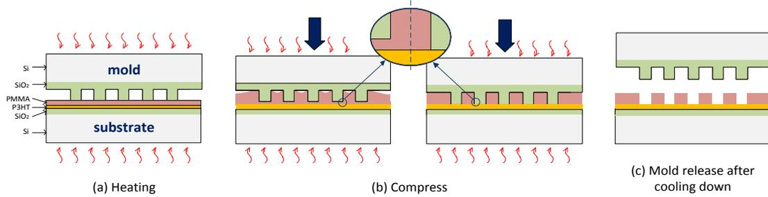
**FIG. 1** Dual-layer thermal nanoimprint lithography process for single-layer patterning.
