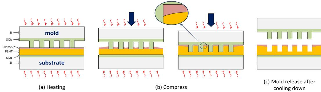
**FIG. 2** Dual-layer thermal nanoimprint lithography process for double-layer patterning.
