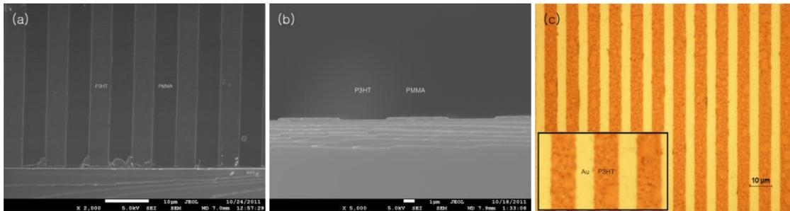
**FIG. 3** Single-layer patterning: perspective view (a), profile (b), and gold pattern after lift-off (c).
