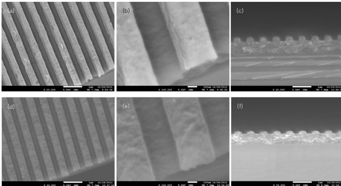
**FIG. 4** Double-layer patterning: PMMA and P3HT pattern (a, b: perspective view and c: profile) and P3HT pattern after removing PMMA by dipping into PGMEA solvent (d, e: perspective view and f: profile)
