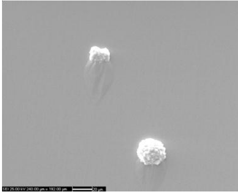
Fig. 1 SEM measurements showing \mu\text{m} -sized cauliflower-shaped epitaxial growth defects (left) and SEM measurements of a quasi crystal pattern printed on a GaN epi-layer. The pattern covers the entire surface despite the growth defect shown to the right. The hole diameter is 90 nm.
