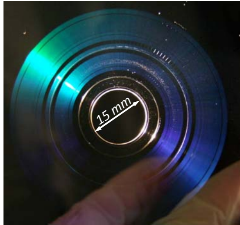
Figure 1: Optical photo of injection-compression-molded replica mold
