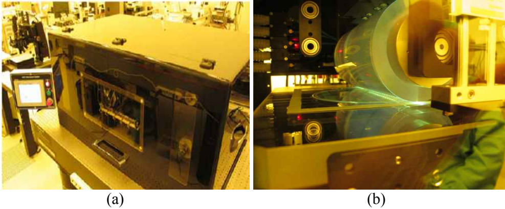
Figure 1: Experimental systems (a) UV-typed roller nanoimprint lithography (RNIL) systems. (b) the adhesion-free transparent roll stamp with length of 210 mm and diameter of 100mm on the RNIL systems. The roll-typed bare material and the replicated h-PDMS mold with width of 300 nm and height of 300 nm are set-up in the roller and mold chucks on the RNIL systems
