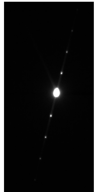
Figure 5: Diffraction from another 50 nm pitch grating which had a lower lithography exposure.
