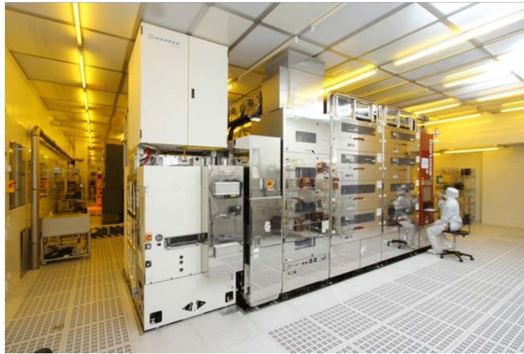
Figure 1 : Outlook on the 1 st Maskless MAPPER-SOKUDO lithography cluster LETI clean room environment
