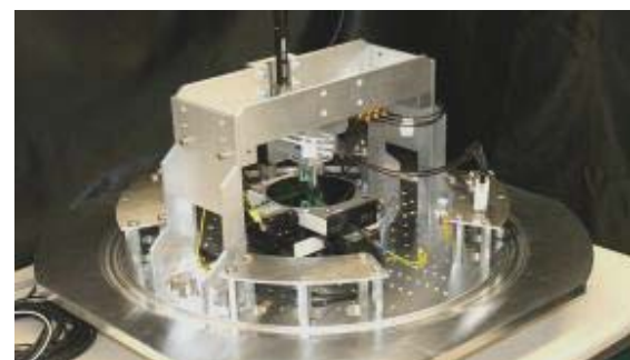
Figure 4. Image of the tool for scanning probe lithography using FN-low-energy electron emission based on 10x10 \mu m scan field top-scanner and 100x100mm bottom-stage for step and repeat operation in closed-loop mode. The same self-actuated, piezoresistive cantilever (see Figure 1) are used for imaging and lithography.
