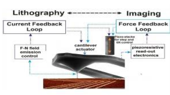
Figure 3. Principle of the Scanning Probe Lithography (SPL) system using a self-development, positive/negative-tone closed loop technique on calixarene-based molecular resist. The same cantilever are used for direct FN-nano-writing, AFM-imaging, pre- and post-imaging (litho-inspection) as well as for pattern overlay alignment.
