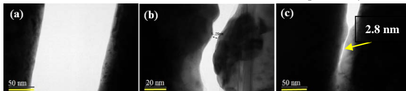
Figure 3. Nano-river reduction using 0.5 \text{ keV} FESEM irradiation with 10 \mu\text{A} emission current setting and probe current setting at 10 position. The narrowing of the nanoriver with 137 \text{ nm} wide before electron beam exposure in (a), after FESEM electron exposures, the \sim 5 \text{ nm} wide nano-channel and the 2.8 \text{ nm} wide nano-stream in the Au dunes were shown in (b) and (c), respectively.
