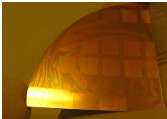
Figure 3: Photograph of microstructures patterned on a quarter 4" Aixtron graphene/Cu wafer.
