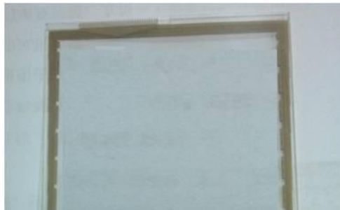
Figure 2. A photograph of screen printed silver electrode on top of patterned metal mesh TCFs in a touch screen sensor.
