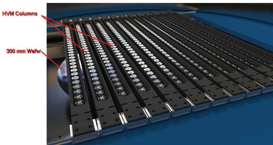
Figure 3: Array of inspection columns arranged over a 300mm wafer
