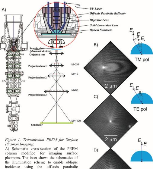
incidence using the off-axis parabolic reflector and normal incidence through the UV objective. The angle of incidence can be controlled from 30-50 degrees by translating the laser beam across the mirror surface. The excited surface plasmons decay to photoelectrons which are then accelerated down the electron optical column and imaged at the scintillator.
