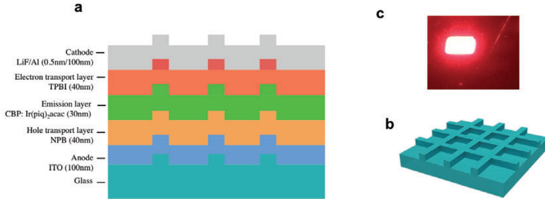
Figure 1: Red Organic Light Emitting Diode (OLED) with nanoplasmonic mesh. (a) Structure schematic: a glass substrate with a nanoplasmonic mesh embedded, a top ITO anode, a back LiF/Al cathode, and in between red phosphorescent organic light-emitting active layers. (b) glass substrate with a nanoplasmonic mesh embedded in it (c) photography of light emission from the fabricated red OLEDs with nanoplasmonic mesh.
