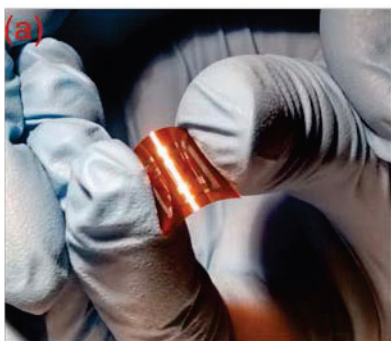
Figure 1: (a) a photo of the CNT FETs fabricated on Kapton film substrates. (b) The liquid gate performance of a CNT FET functionalised with the E2 aptamer, before and after E2 exposure.
