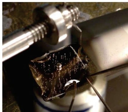
Figure 3: Bubble generation during water electrolysis
