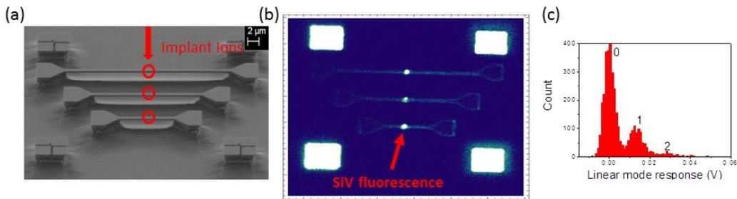
*Figure 2:* (a) SEM image of the diamond nanobeams (fabricated at Harvard) showing the implant locations. (b) Photoluminescence of the nanobeams after ion implantation showing the spatial location of the implanted ions relative to the nanobeams (c) Histogram of an *in-situ* diamond detector response showing quantized single ion detection for 200 keV Si ions with an average of 1 ion per pulse, demonstrating low energy single ion detection in diamond.
