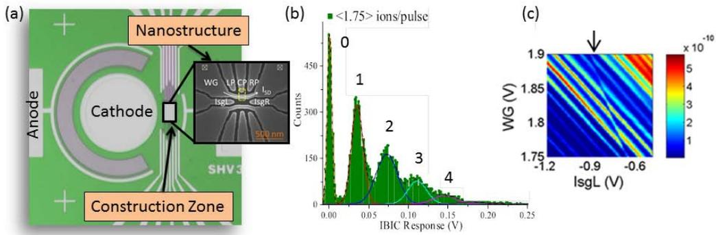
*Figure 1:* (a) Optical image of the integrated *in-situ* single ion detector and SEM of the nanostructure for low temperature transport. (b) Histogram of the detector response showing quantized single ion detection for 200 keV Si ions with an average of 1.75 ions per pulse. (c) Low temperature transport data taken on a counted implant sample, the charge offset shown is likely due to an electron tunneling between the electrostatically formed SET and the donor.
