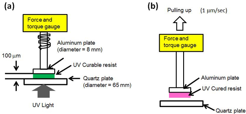
Figure 1. Schematic measuring systems for (a) dynamic modulus and stress of UV curable resist and (b) release force and strain of cured resist.
