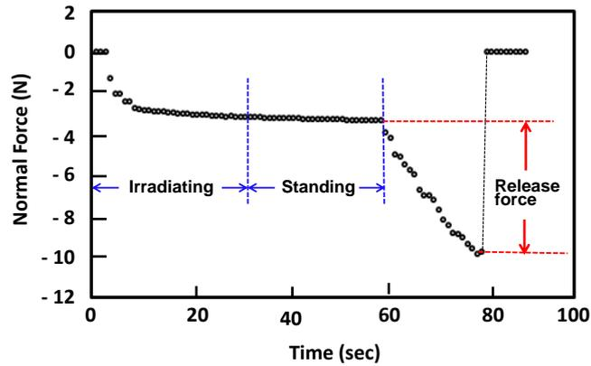
Figure 2. Normal force (NF) change profile for UV curing and demolding process. Resist: PAK-01 (100  $\mu\text{m}$  thick).
