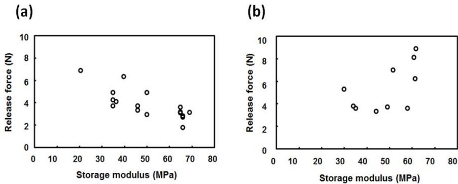
Figure 3. Relationship between release force and storage modulus of UV cured resist. Mold: (a) quartz plate with plain surface and (b) quartz plate with patterned surface ( $L/S=6/2 \mu\text{m}$ , line height= $1.2 \mu\text{m}$ ). Resist: PAK-01 (100  $\mu\text{m}$  thick).
