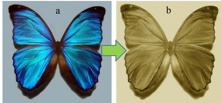
Figure 1: Illustration showing the conceptual conversion of natural Morphos butterfly wing is converted into gold wings. (a) The real morphos butterfly. (b) The electroplated butterfly with Au.
