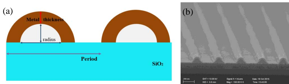
Figure 1(a) Schematic diagram of arch metal structure (b) SEM image of bilayer resist profile after developing process.
