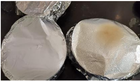
Figure 2. Picture of the perovskite reaction occurring in the coaxial fibers after electrospinning as residual solvent evaporated. A fiber mat immediately after spinning (left) the reaction occurs in a fiber mat five minutes after processing (right).
