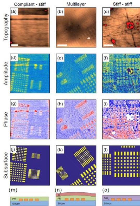
Figure 1: Surface and subsurface probe microscopy of several samples. The surface topography does not reveal any information about the buried features and the subsurface probe microscopy resolves the buried features. This concept is being developed for wafer alignment and overlay on product features (patent pending).
