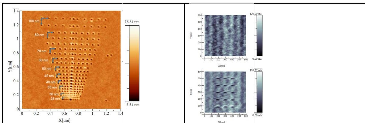
Figure 2: Left: nanopatterning of contact holes on a metal resist with various pitches. Right top: subsurface image of buried lines. Right bottom: nanopatterned contact holes, aligned by subsurface probe microscopy on top of the buried lines and fabricated with the SPM tip.
