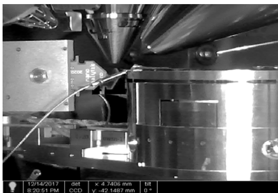
Figure 2: Left Image of AFMinSEM (Nanoanalytik GmbH) system showing the active cantilever and the SEM column; Right Fowler-Nordheim-plots of the field emission from a diamond tip for two different tip-to-sample distances.
