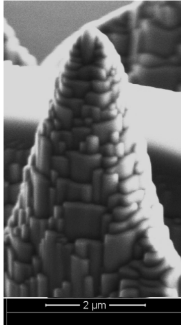
Figure 1: Processed diamond tip after micro-machining with a focused Ga + ion beam
