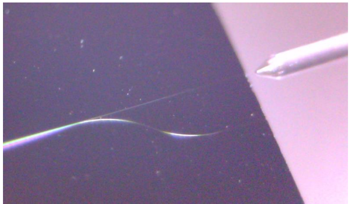
Figure 2: Characterization of prototypes showing cleaved edge with waveguides and lensed optical fiber.
