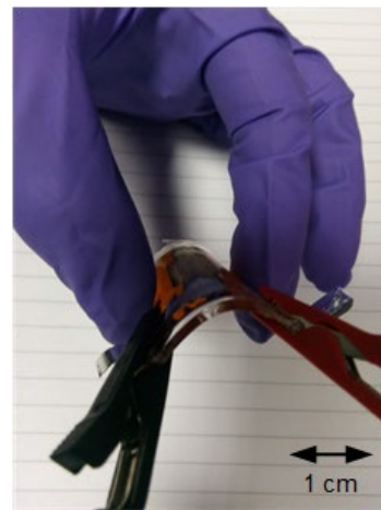
Figure 3: Bending test on device fabricated on Kapton substrate.
