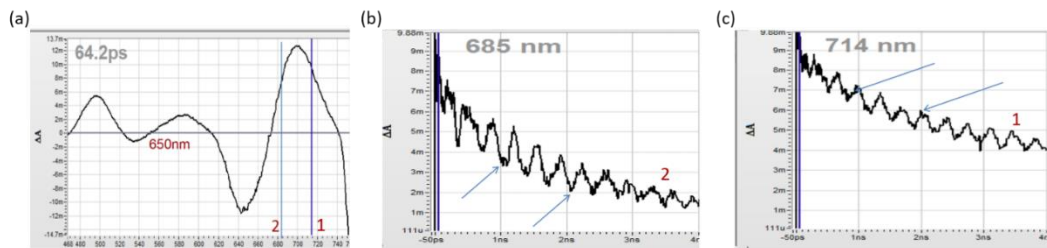
Figure 3. (a) Broadband transient absorption spectrum (b) Time-dependent absorption spectrum at 685 nm wavelength. (c) Time-dependent absorption spectrum at 714 nm wavelength.
