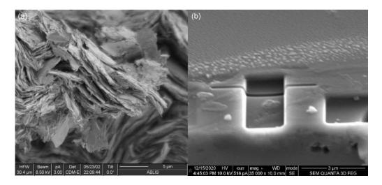
*Figure 1: Imaging and milling experiments taken by our Rb FIB:* (a) A secondary electron image of a pencil lead sample by Rb ions. The image is acquired under 8.5 keV working voltage and 2 pA beam current. The resolution of the image is around 30 nm. (b) The image shows a box pattern milled by  $Rb^+$  ions under 8.5 keV, with a burn line by  $Ga^+$  to illustrate the milling depth.
