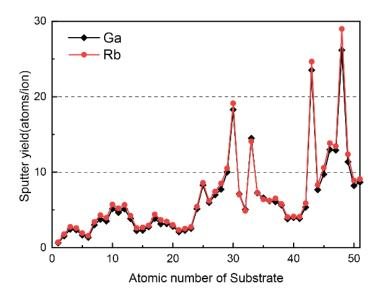
*Figure 2: Sputter yield simulation by SRIM:* This figure plots two curves of  $Ga^+$  (in black) and  $Rb^+$  (in red) predicting the milling ability over various substrate. The energy of ions is set to 10 keV, and each simulation applies 10000 ions in total. The result shows our  $Rb^+$  performs a better ability on sputter yield than  $Ga^+$ .
