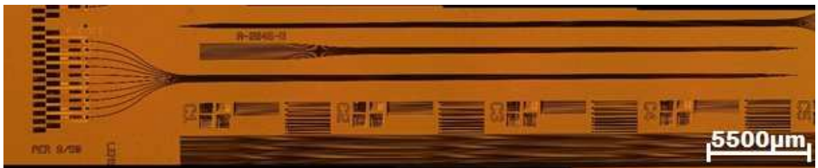
Figure 2: Overview of optical waveguide probe on substrate wafer: The structure starts from the left-hand side with bond pads for laser diode chip integration and ends on the right-hand side with the optical outcoupling structures to be placed in the cochlea.
