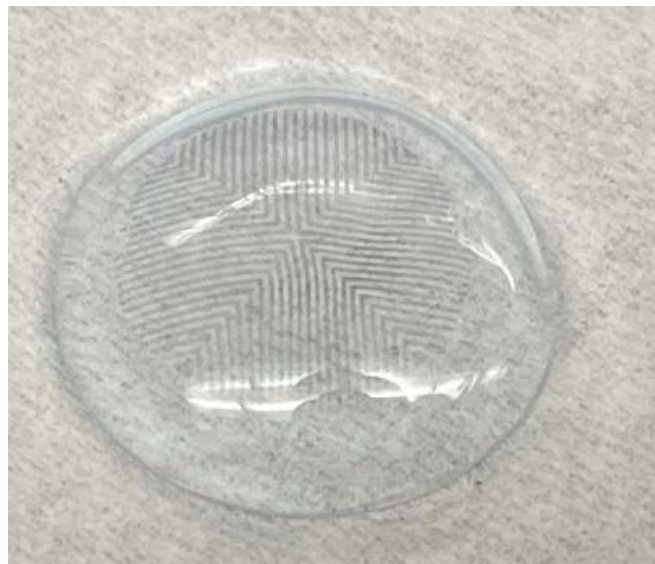
Fig.2 Photograph of a representative contact lens coated with densely arranged Ti lines of 100 \mu m width and spacing
