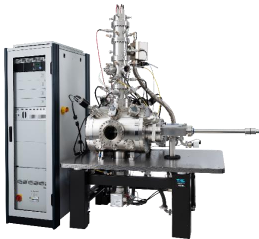
Figure 1: Q-One system (Ionoptika Ltd.) high-resolution Focused Ion Beam system, equipped with a piezo-driven stage allowing for precise and repeatable positioning. Load-lock provides high vacuum level in the main chamber while enabling sample exchange.
