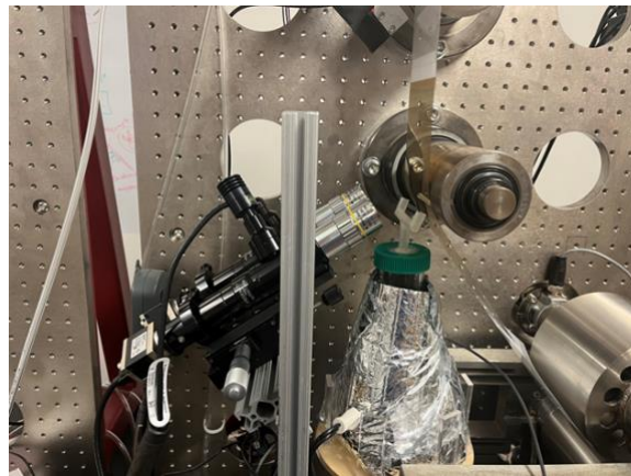
Figure 1. Experimental setup for imaging condensation.
