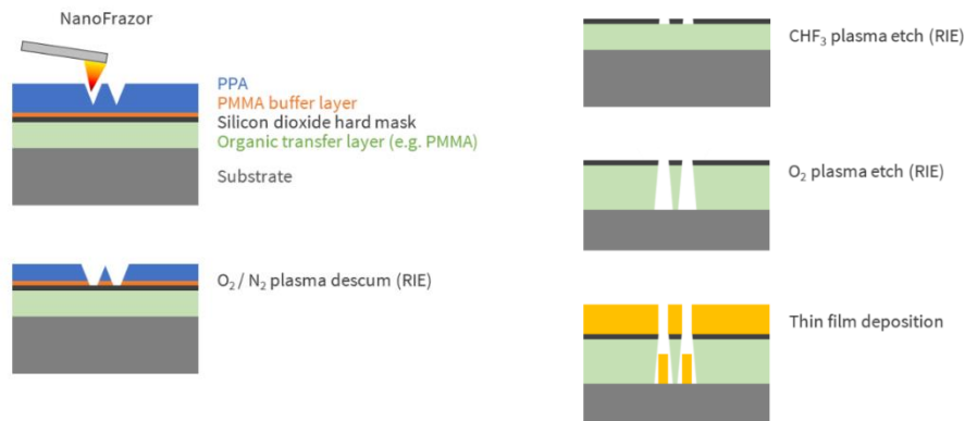
Figure 2: Process flow of high-resolution lift-off with the NanoFrazor.
