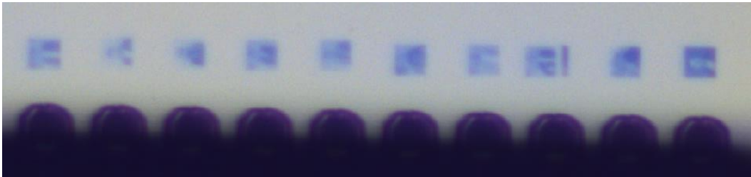
Figure 2: Same array of thermal cantilevers as Figure 1 under the NanoFrazor microscope, with different designs written by each 50microns away from the tip for demonstration purposes, micrograph with 20x magnification
