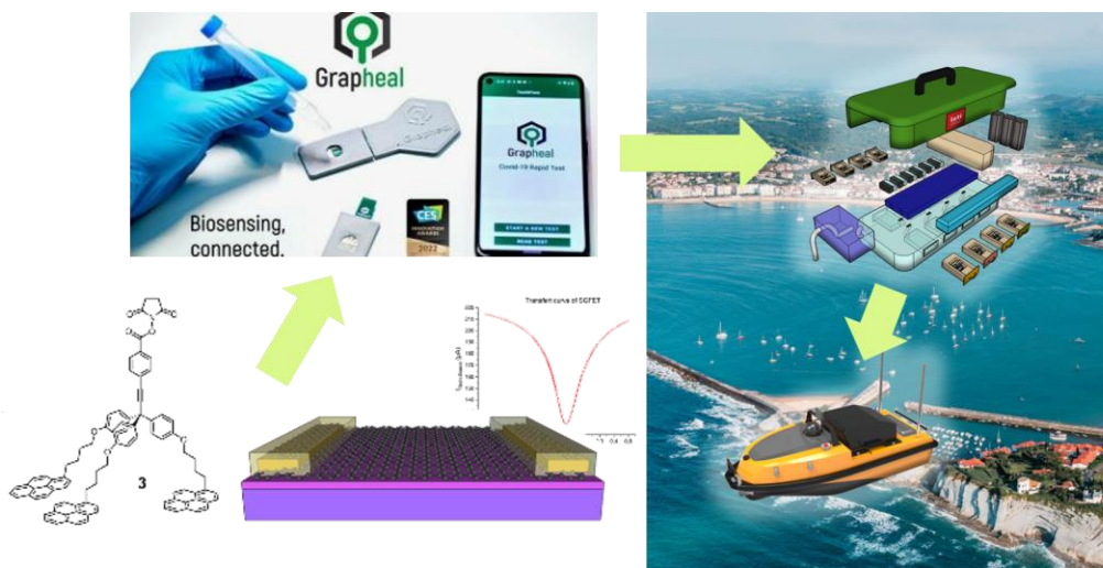
Figure 1 : Composite illustration of the comprehensive process of deploying graphene-based biosensors for environmental monitoring. The wirelessly operated commercial grade SGFET developed by Grapheal. The state of the art non-covalent functionalization protocol we rely on to ensure specificity for the biosensor. Depicted on right hand is the deployment in a coastal setting, where autonomous vessels carry the biological analysis system that unlock effective real-time water analysis with graphene sensors.
