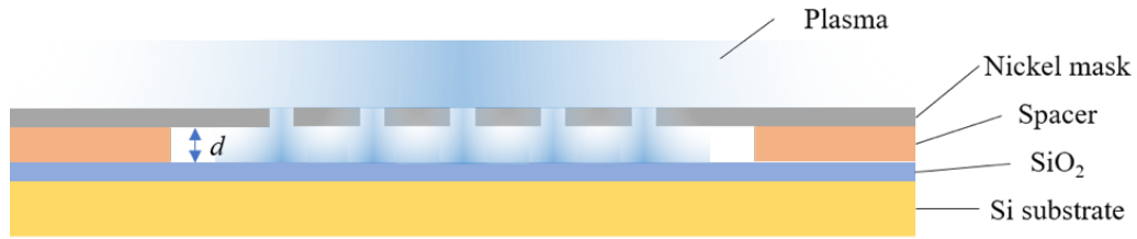
Figure 1: The shadow mask plasma etching schematic.
