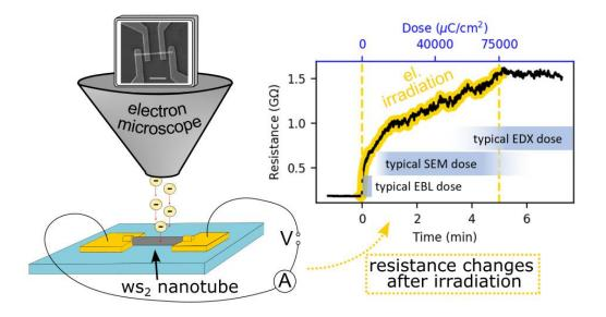
*Figure 1:* Schematic illustration of the electron irradiation experiment and its results. The resistance of a nanotube device increases rapidly within first seconds of electron irradiation. Reprinted from: Kovařík M. et. al, *ACS Appl. Electron. Mater.* 2024 6 (12), 8776-8782.
