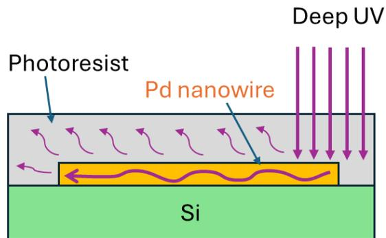
Figure 2: The DUV plasmonic waveguiding effect responsible for the unexpected photoresist exposure on top of the Pd nanowire arrays.
