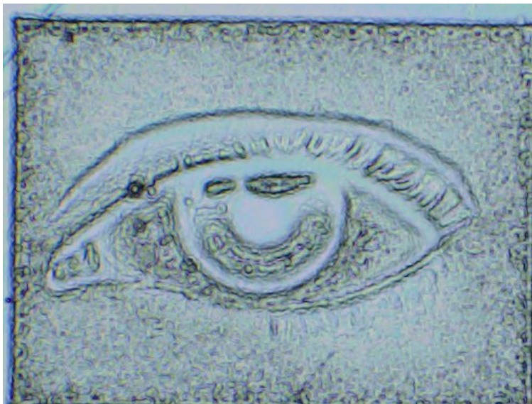
Figure 2: Grayscale contact i-Line lithography using carbon mask. AZ4330 resist (image flipped for comparison to mask).
