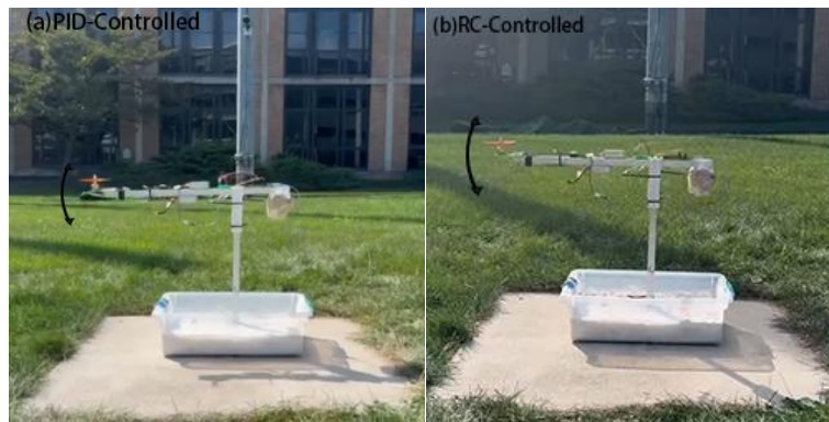
Figure 2 Photo of the testing rig for the motor-driven lever balancing test. (a) PID control test. (b) RC control test.
