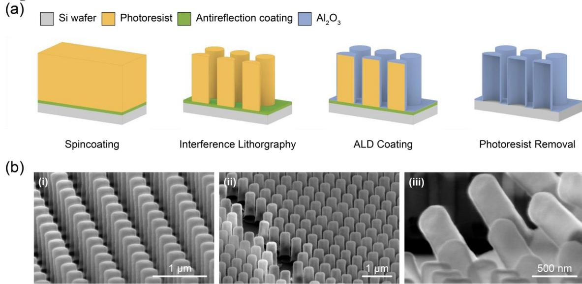
**Figure 1.** (a) Schematic illustration of the fabrication process for the thin-shell nanopillar array. (b) SEM image of the fabricated thin-shell nanopillar array, demonstrating high uniformity and periodicity. (i) Before template removal. (ii,iii) After template removal.
