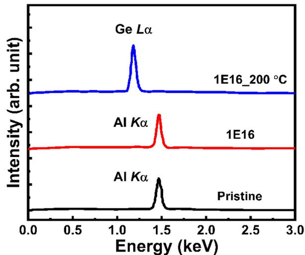
**Figure 4:** EDX spectra of *p*-Al/*a*-Ge (pristine), irradiated with 1000 keV Xe<sup>+</sup> ion at a fluence of  $1 \times 10^{16}$  ions-cm<sup>-2</sup> and irradiated at a fluence of  $1 \times 10^{16}$  ions-cm<sup>-2</sup> followed by annealing at 200 °C
