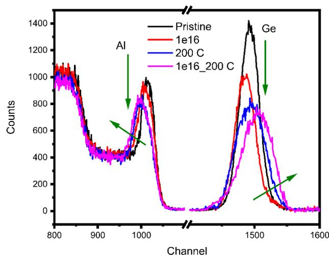
**Figure 2:** RBS spectra of *p*-Al/*a*-Ge (pristine), irradiated with 1000 keV Xe<sup>+</sup> ion at a fluence of  $1 \times 10^{16}$  ions-cm<sup>-2</sup>, annealed at 200 °C and irradiated at a fluence of  $1 \times 10^{16}$  ions-cm<sup>-2</sup> followed by annealing at 200 °C
