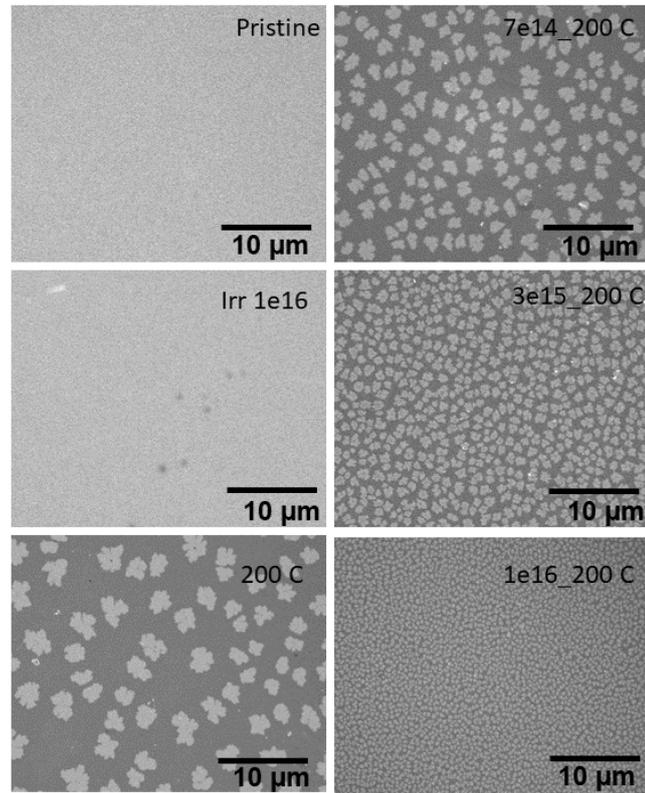
**Figure 3:** FESEM image of *p*-Al/*a*-Ge irradiated with 1000 keV Xe<sup>+</sup> at a fluence of  $1 \times 10^{16}$  ions-cm<sup>-2</sup>, annealed at 200 °C, and irradiation with different fluence  $7 \times 10^{14}$ ,  $3 \times 10^{15}$ ,  $1 \times 10^{16}$  ions-cm<sup>-2</sup> followed by annealing at a fixed temperature of 200 °C
