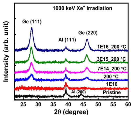
**Figure 1:** XRD data of *p*-Al/*a*-Ge irradiated with 1000 keV Xe<sup>+</sup> at a fluence of  $1 \times 10^{16}$  ions-cm<sup>-2</sup>, annealed at 200 °C, and irradiation with different fluence  $7 \times 10^{14}$ ,  $3 \times 10^{15}$ ,  $1 \times 10^{16}$  ions-cm<sup>-2</sup> followed by annealing at a fixed temperature of 200 °C
