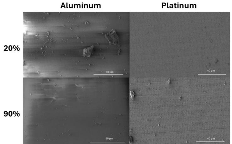
**Figure 1.** (a) SEM of nanostructures. (b) SEM image of Pt and  $\text{Al}_2\text{O}_3$  samples tested at 20% RH & 90% RH
