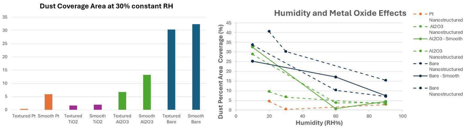
**Figure 2.** (a) Bar chart of coverage area for different samples at constant 30% RH. (b) Plot of dust surface area coverage at varying humidity levels. Substrates have a variety of surface coatings to alter conductivity and nanoscale roughness. RH% levels were captured for  $\text{Al}_2\text{O}_3$ , Au, Pt and bare.
