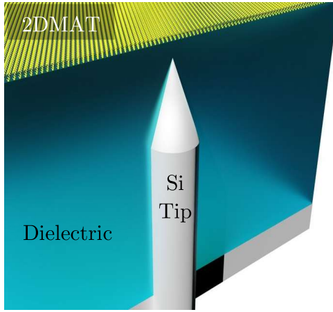
Figure 1 Schematic representation of a 2DMAT-Tip system
