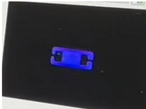
Figure 2: The continuous illumination of an LED driven by an electron beam was captured using a CCD camera through a coaxial optical system.
