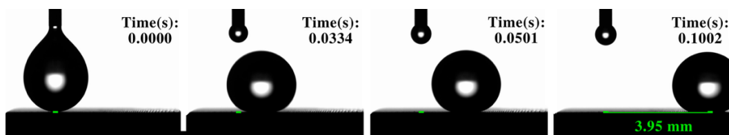
Figure 2: Droplet motion on coating-free Al wetting gradient (green line between start and finish locations is 3.95 mm).
